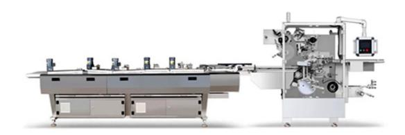
SL-SBSM250 series packing machine is specially designed for the packaging of high-end chocolate, wafer chocolate, and wine heart truffle products, the single twist with cold sealing then paste the iconic strip, with good sealing, and strong identification characteristics.
