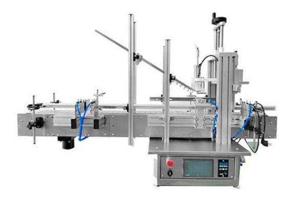
This tabletop cork pressing machine is suitable for bottle caps of different sizes. The capping chuck can be customized according to your need. It is with an automated cork feeder, which enables it to press corks rapidly. The machine can be widely used in pharmaceutical, cosmetic, beverage, wine industries. Help to save labor and improve work efficiency.
