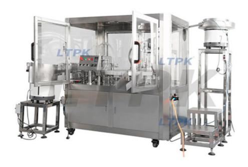
This machine is a specialized equipment in the sampling tube and detection reagent bottle filling production line. It adopts a rotary tracking filling method, which ensures stable filling and high production capacity. Adopting PLC touch screen control, ceramic pump filling, disc positioning upper cover screw cap, high filling accuracy, reasonable design, easy operation and maintenance.
