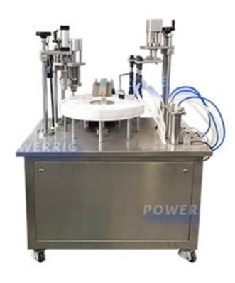
It includes one working disk and two vibrating plates. It has 3 filling heads and 16 positions. It is mainly used for filling and sealing glass bottles perfume.
