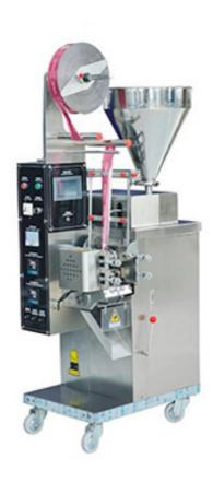
The machine is suitable for automatically packaging of viscous products with free-flowing such as shampoo, lotion, edible oil and broth, etc. The integrated processes of bag making, measuring filling, sealing cutting, counting and hot pressing codes can be done automatically. Packing material include several kinds of heat seal lamination, such as PET/plated AL/PE, PET/PE, PAPER/PE, NYLON etc.
