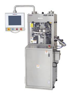
Lab Press – PILOT 200 DL is a High Tech Double Layer & Mono layer Rotary Tablet Press is essential for R & D and small batch production. This Single sided R & D Double Layer Tablet Press fully conforms to GMP and the safety requirements, featuring versatility with a quick change of tooling.
