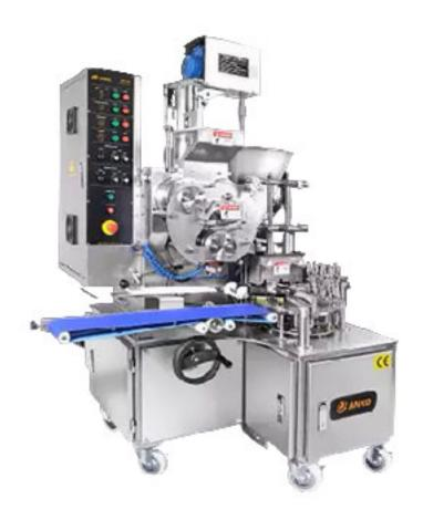
Automatic Wonton Machine completes the process of making wonton after putting in prepared dough and stuffing. The texture of stuffing stays the same from beginning to end; the pinched pattern on top is as beautiful as hand-made one. The final products show that ANKO is highly concerned with quality control.
