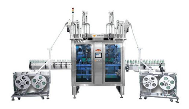
DSVC-EB II is a high speed double-heads sleever applicator machine. When two heads operate simultaneously, the maximum production speed is up to 600bpm/180mm label length.
