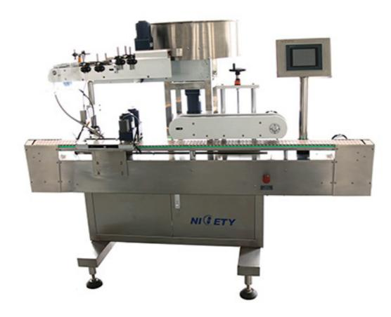
Used for plastic caps feeding, sorting, dropping and capping automatically.
