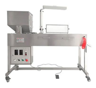
JYG-220 drug inspection machine, it can capsules and tables (pills), by adding in conveyor rooler feeder even fall in conveyor roller, drugs, at the same time, along with the flip on the move, conveyor roller for artificial detection, picked out the unqualified products. The machine in accordance with GMP standard, check drug no dead Angle blind spots, is the capsules and tablets (pills) agent appearance test, in order to achieve the ideal equipment for drug qualified.
