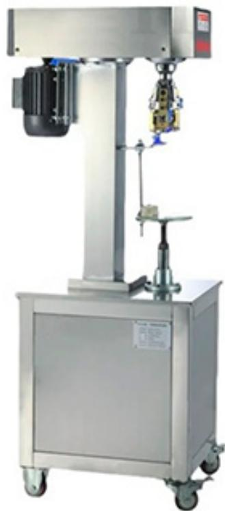
The Semi-Automatic Electric Oral Liquid Aluminum Cap Crimping Machine. This device is designed for sealing aluminum caps onto glass or plastic vials, commonly used for oral liquid packaging in the pharmaceutical and healthcare industries. Here's a description of its features and functionality:
