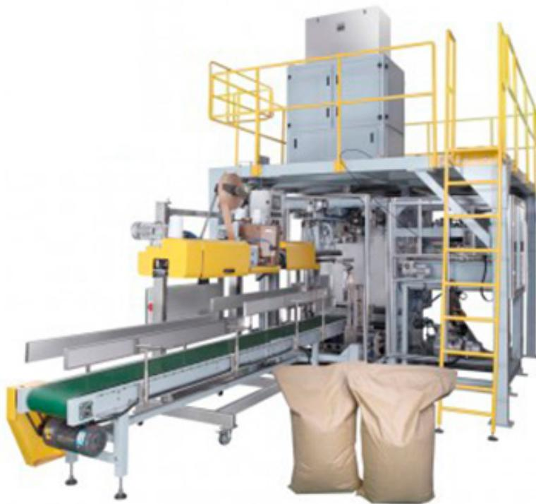
ZD-D system auto granule bulk bag packing machine is developed specifically for 10~15 kg heavy bag of granule products which made in agriculture and food industry, such as rice, seeds, fertilizer, feed, sugar, pet food, etc. This machine can realize automatic weighing, bag-feeding, filling, bag-conveying, sealing/sewing, etc. Our company new improve the technology, using high speed servo weighing machine instead of normal weighing machine, increase the weighing speed by a large margin.
