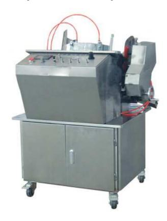
The machine can print letter on empty hard capsule, filled capsule, soft capsule and tablets of various shapes and specs.
