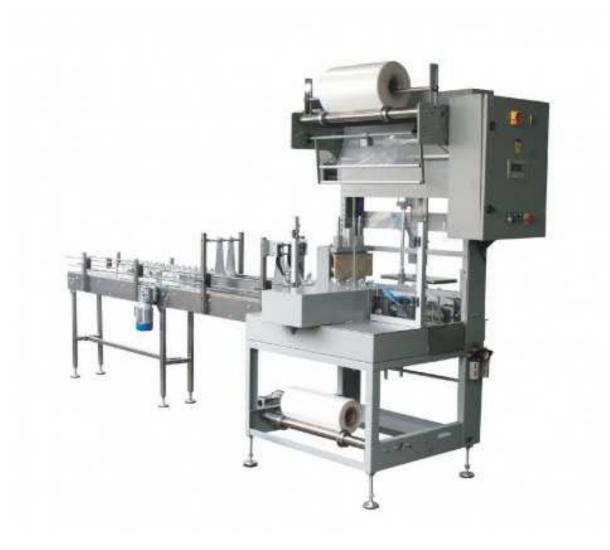
Shrink wrap machines apply heat to shrink a plastic film around a product. This process is often done by automated equipment, but manual and semi-automatic shrink wrap machines are also available. Shrink wrap machines cover the item, and then sent it through a heat tunnel or oven for shrinking.
