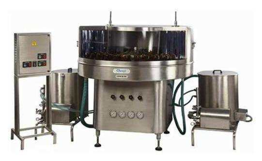
Rotary Bottle Washing Machine is compact and highly efficient machine with elegant look. This multifunctional multi featured machine meets the GMP requirements of washing for glass and plastic bottles. The machine operates on the rotary principle with "GENEVA" mechanism and requires manual loading and unloading of bottles.
