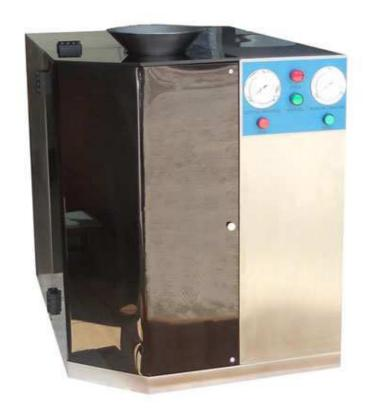
In the relatively airtight environment-working cabin, use high and low pressures to alternate changes rapidly "pressure shear" causing pulsed drawing force to the capsule. Under the continuous function of the pulsed drawing force, the capsule is gradually drawn and separated.
