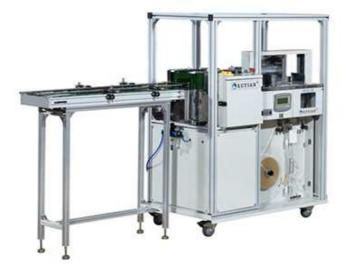
The WK04-30AM10 Automated Banding System will bring ease to your packaging line by neatly banding your small boxes / packages in easily handle able bundles. The WK04-30AM10 uses a dual conveyor belt setup to automatically stand boxes / packages up and accumulate them into the automatic pusher. The pusher then feeds the boxes / packages into the banding machine and applies a nice secure band.
