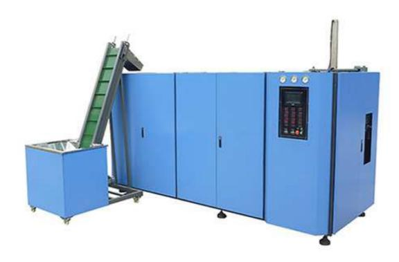
GF130-2A two-step manually preform inserted full-auto bottle blower is applicable for blowing the carbonic acid beverage bottle, mineral spring water bottle, farm chemical bottle, oil bottle, medical, hot-filled bottle in any shapes and made of PET, PC, PP or PE raw material.
