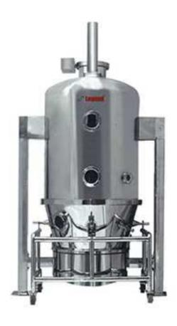
Fluid Bed Dryers (FBD) are primarily used in almost all chemical, pharmaceutical, food, dyestuff and other process industries to dry materials by fluidization with hot and / or dehumidified air, which creates a turbulence in the wet product (not totally liquid) while flowing through it.
