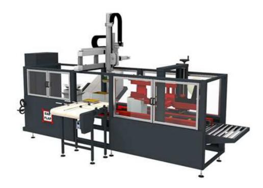
The Model BPP550 3 in 1 Auto Case Erector, Sealer and Filler is an innovative, 3 in 1 automatic carton erector, carton sealing and carton filling machine developed by innovative Spanish company Ear-Flap. It is capable of handling cartons up to 530 mm length, 310 mm width and 500 mm height. It utilises adhesive tape to seal the carton. It comes standard with a PLC and LCD color touch screen control panel. It can achieve outputs of up to 10 cartons per minute.
