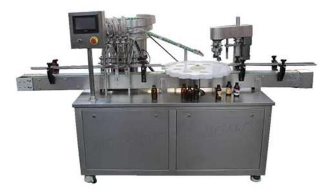
This filling sealing machine is suitable for: Syrup, oral liquid, E-liquid, Eye-drops and Ear-drops into various round and flat Glass bottles with the range from 10-50ml.
