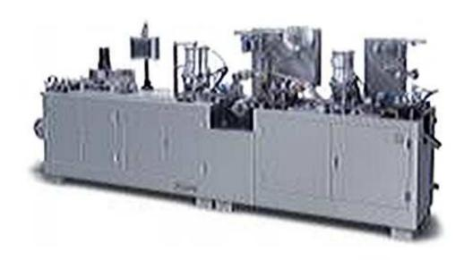
DPR-160A Tropical (ALU/PVC/ALU) Blister Packager is the innovation product in China and got two patents of the state. It can be used for three packing kinds for ALU/PVC, ALU/ALU, ALU/PVC/AVC and up to the purpose that a machine with three usages just to change moulds.
