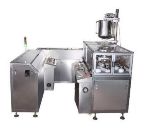
SED-3SJ type automatic suppository production line is suitable for the production of special shape such as bullet head, torpedo shape and duck bill, which satisfies the production of various suppositories. (according to the specifications of the mould according to the requirements of the customer)
