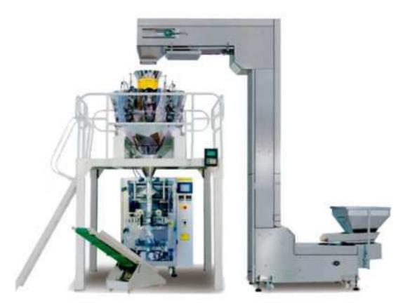
Automatic form-fill-seal packing machine explores the roll of film to make bags of pillow bags, gusseted bags. The maximum film width is 600mm. Loading weather can be added which is up to 3kg. It can automatically realize bag making, filling, printing, sealing, gusset making, hand hole making etc.
