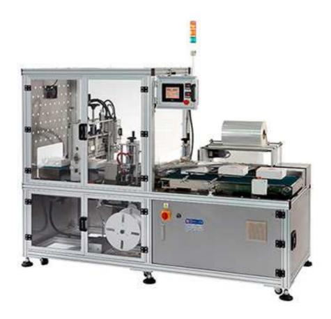
Auto Side Sealing Machine, standard model USA-004B can adjust its packaging height basing on product to have strong seal & nice look. USA-004B adopted constant heating sealing knife by SSR control to keep stable temperature, power saving and easy change. POF is recommended to work with. USA-004B can reduce the film wastage & seal multiple length without any limitation. Simple design, easy operation, film saving & high efficiency, it is the latest model of wrapping machine.
