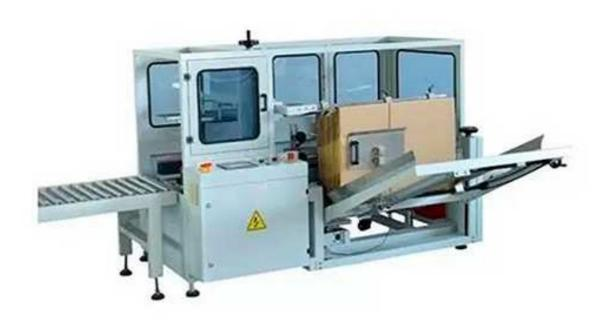
Automatically finish the process of opening, molding, filling, packaging and sticking tape for the cartons.
