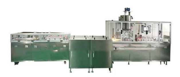
SP-15L type automatic suppository production line is suitable for the production of special shape such as bullet head shape, duck mouth shape and other shapes, which satisfies the production of various suppositories. (according to the specifications of the mound according to the requirements of the customer).
