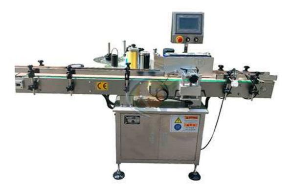
Suitable for drinks, food and other industries have localization features or bottles is bigger and heavier round bottles make circular orientation labeling requirements, can stick a double standard at the same time.
