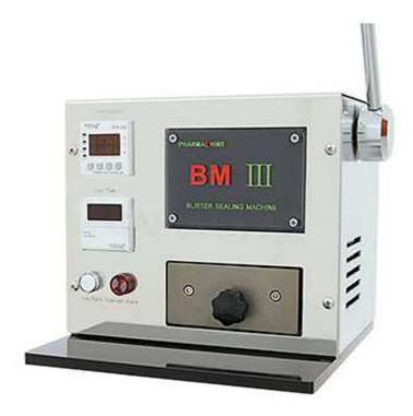
BM-III blister packing machine is designed for small pharm factory, healthcare plant, food plants and preparation rooms, which can be used to pack solid drugs like a capsule, tablet, gelatin pearl, suppository, milk tablet, candy, and hardware.
