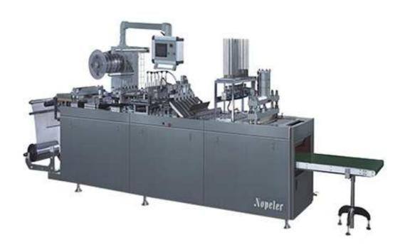
The equipment can automatically complete Blister forming, Blister Die cutting, Blister transiting, paper-card dropping, heat sealing, and output delivery and other functions.
