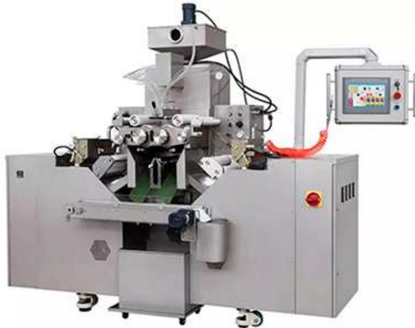
Our softgel encapsulation machine is used for producing all kinds of soft capsules with different size, shape and color.
