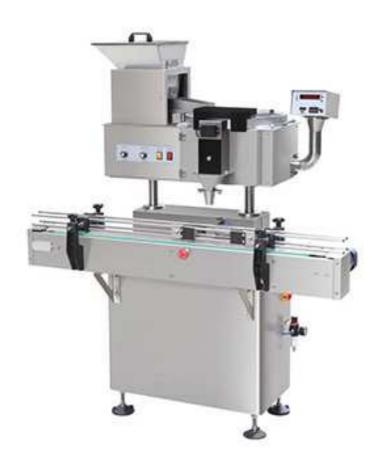
Auto-photoelectric counting packing machines used be electromagnetic vibration plates, the motor drive discs rotate to automatically bring the drug into the bottle. It is convenient and fast to replace the counting disks of different specifications and models, without another adjustment. Auto-photoelectric counting packing machines is the advanced, attractive appearance, and economical bottled and bagging equipment in counting machinery.
