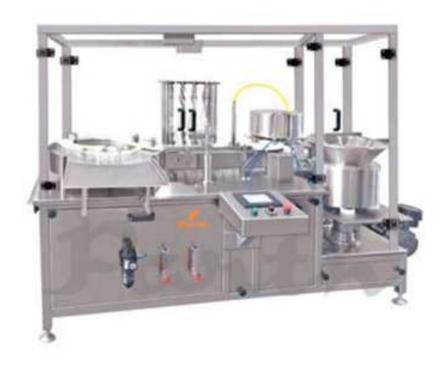
Automatic Volumetric Liquid Vial Filling Machine works on volumetric principle with diving nozzles. The unit is made compact, versatile and enclosed in stainless steel elegantly matt finish body, consists of S.S. Slat Conveyor, Reciprocating Nozzle with self-centering devices & SS Syringe. No container No filling system arrangement is standard features of the machine. The main drive of the machine and conveyor drive consist of A/c Motor with synchronized variable A/c Frequency Drive.
