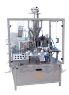
Automatic Single head tube filling machine is precision built on sturdy welded MS frame completely enclosed in stainless steel sheet and doors are providing to facilitate the servicing of machine.
