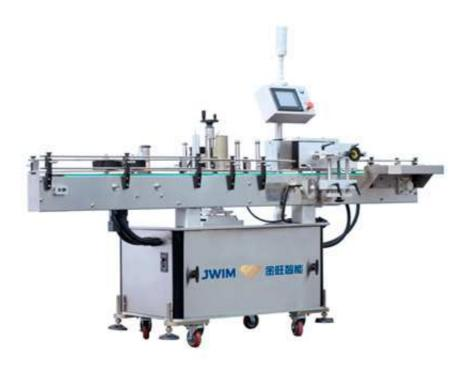
TN-150AS Intellectual Labeling Machine is controlled by the PLC, HMI and servo drive labeling. The machine is easy to operate and has helping function and fault indication function. It is suitable for the self-adhesive labeling of round bottles
