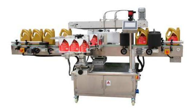
TS-150 self adhesive labeling machine is widely used for the square, flat bottles labeling in agrochemical, chemical and other industries. It has the features of advanced technology, simple operation, and compact structure. It uses sensor inspecting, PLC control and touch screen. Conveying, bottle separating are inverter speed adjusting.
