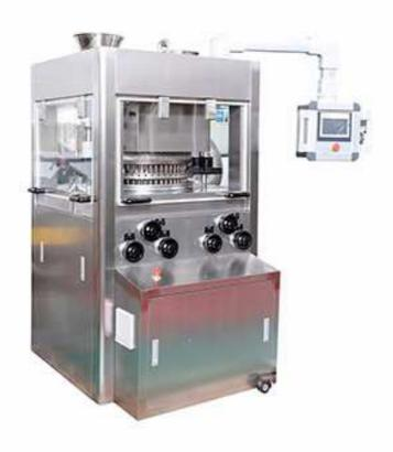
The High Speed Rotary Tablet Press Machine with Good Price has a fast rotation speed, high output, and good tablet quality. Double pressure is used for tableting, they are all controlled by microcomputer, which can continuously compress granular materials.
