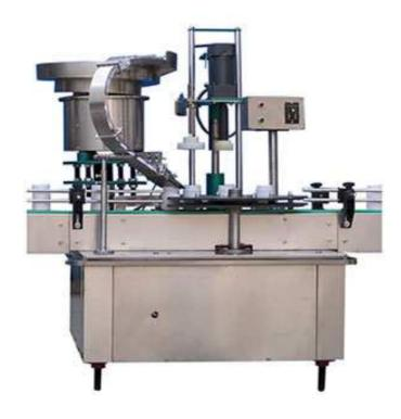
DXG automatic single head capping machine is mainly used for screw caps of various round plastic caps, aluminum caps, and iron screw caps screwing. It is an ideal bottles capping machine in the food, pharmaceutical, cosmetic, pesticide, cosmetics and other industries.
