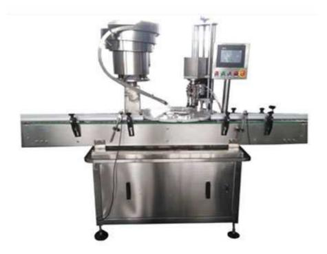
SP-SG automatic locking capping machine is designed with special structure for screw sealing. Three-knife sealing has stable operation with good sealing feature. This machine adopts frequency converter controlling, transmission mechanism applying cam principle, disc divider positioning, easy operation, stable and reliable operation. Capping does not hurt lids, capping heading easy to dismantle. The different lids can be adjusted and can be used universally.
