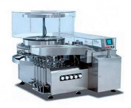
QCL series automatic washing machine consist of in feeding section, ultrasonic treatment section and final washing section, the containers are going through those sections for completion of the whole washing processing by Ultrasonic treatment, prewashing and final washing steps, the cleaning quality of the container washed meets any Pharmacopoeia and being able to validate.
