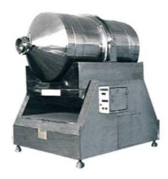
EYH Series Tow dimensions mixer mainly consists of three big parts, rotating cylinder, swinging rack and frame. The rotating cylinder lies on the swinging rack, supported by four wheels and its axial fixation is done by two stop wheels. Two of the four wheels are driven by rotating system to make the cylinder rotate. The swinging rack is driven by a set of crankshaft swinging bar which is mounted on the frame and the swinging rack is supported on the frame.
