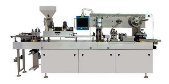
This machine uses forming material to contact heating, press forming (thickened ALU-ALU), plank pose sealing advanced function, according to GMP standard. Suitable for medicine (tablet, capsule, amouples, cylindriod vials, pill, suppository), food, industry, cosmetic and medicine device etc.
