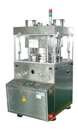
This machine is a double-press type continuous automatic tablet press for pressing granular raw materials into tablets. It is mainly used in pharmaceutical industry and also the chemical, food, electronic industries.
