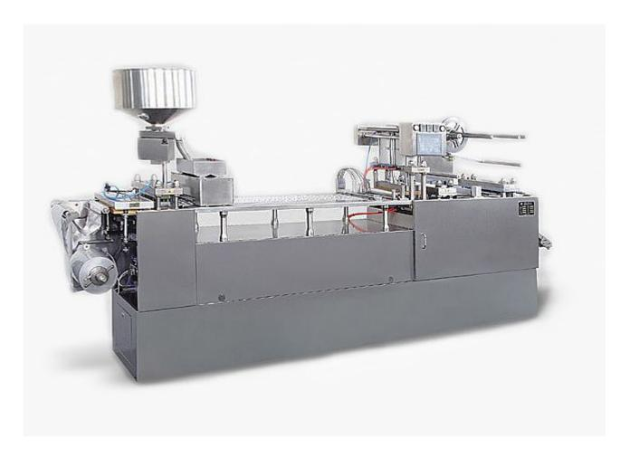
This machine adopts PLC Human Interface, frequency speed regulation, high automation, easy operation. It integrated with hard Alu (PVC) forming, Automatic Feeding, PTP sealing, batch number printing, perforation, cutting, waste winding. It conforms to "GMP" requirement, suitable for Alu/Alu, Alu/Pvc, Pvc/Paper package.
