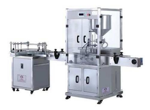
The Automatic cream filling machine is very important equipment for cosmetic production. The machine can be designed according to the capacity. It can use with the bottle Unscrambler, capping machine and labeling machine, to form a complete production line.
