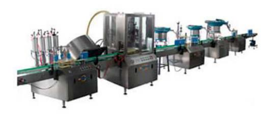
2800B automatic aerosol filling machine consist of can arrange machine, rotary liquid filling machine, valve insert machine, rotary sealing and gas filling, automatic weight checker, water bath, nozzle presser, cap presser, ink jet printer, carton sealing & strapping machine.
