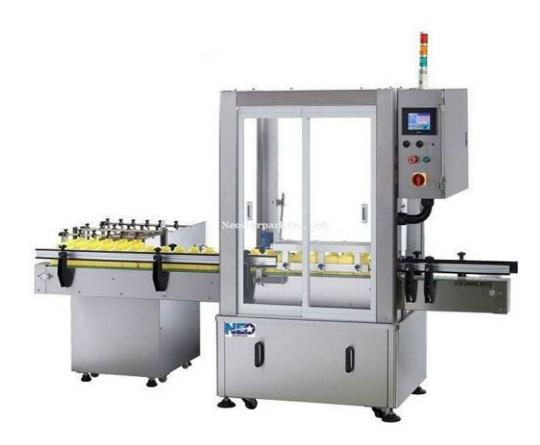
Automatic Bottle Rinser NBW-565 is built to help with product security and sanitation. Air blowing to bottles after bottles inverted and dust will be removed by vacuum. It can suits for any material of bottles and especially designed for integrating with exist conveyor or packaging system.
