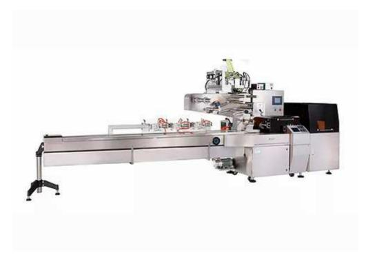
The box motion design of this machine gives longer seal times, resulting in much stronger seals.
