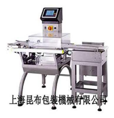
The machine is suitable for checking the weight of the products. The machine can reject the substandard products automatically.
