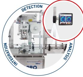
Utilising sophisticated analysis algorithms, the **SealPro Total** provides real time integrity monitoring of every single package or container on the packaging line – at the speed of the machine throughput.
